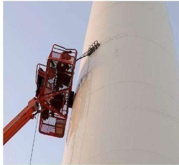
In-service Inspection of windmill tower weld using ToFD & PAUT with fully automatic scanner For Siemens Gamesa Renewable Energy (SGRE)
