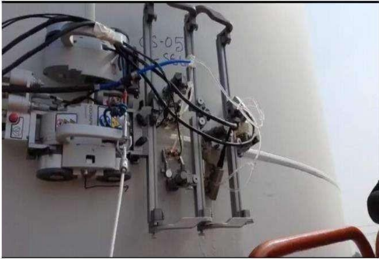
In-service Inspection of windmill tower weld using ToFD & PAUT with fully automatic scanner For Siemens Gamesa Renewable Energy (SGRE)
