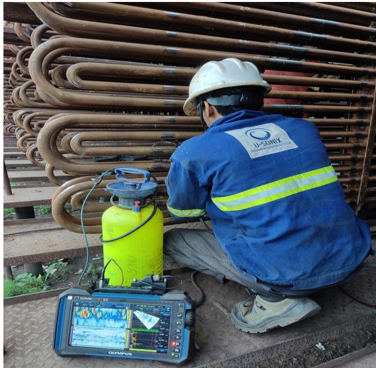
Boiler Tube Inspection at TATA Power, Jamshedpur, India
