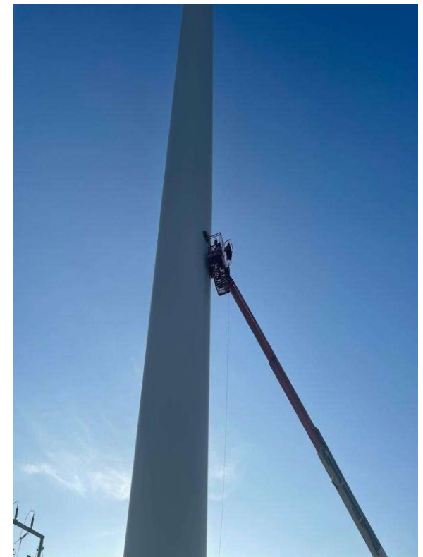
Inservice Inspection of windmill Tower Using SteerRover for SGRE in Bijapur, India
