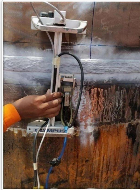
PAUT Inspection at ONGC Offshore Platform
